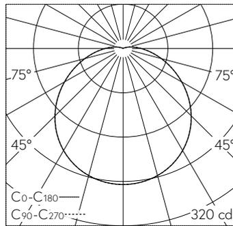
LED 3000 K 8.1 W 936 lm-h / CIE Flux 42 72 90 96 100 / A30 selon DIN 5040
