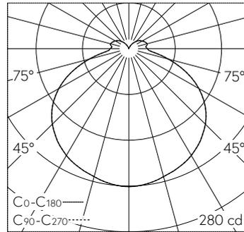
LED 4000 K 10.2 W 946 lm-h 130°/130° / CIE Flux 39 70 90 85 100 / B31 selon DIN ...
