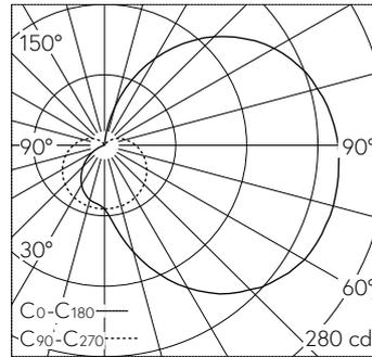
LED 3000 K 11.7 W 936 lm-h / CIE Flux 23 49 74 61 100 / B11 selon DIN 5040
