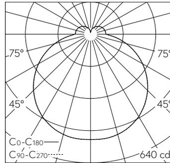
LED 3000 K 28 W 2348 lm-h 128°/128° / CIE Flux 39 69 88 82 100 / B31 selon DIN 5...
