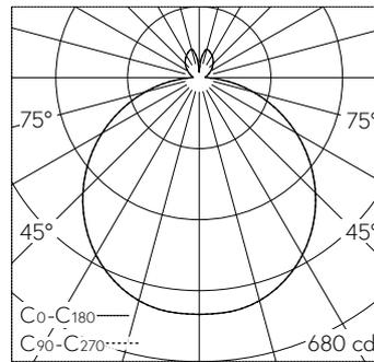
LED 3000 K 18.5 W 1950 lm-h / CIE Flux 45 76 93 89 100 / B43 selon DIN 5040
