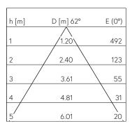
LED 3000 K 11.8 W 537 lm-h  $62^{\circ}$  / CIE Flux 84 97 100 100 / A70 selon DIN 5040
