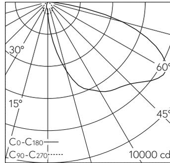
LED 3000 K 70.2 W 8750 lm-h / CIE Flux 34 70 94 100 100 / A30 selon DIN 5040
