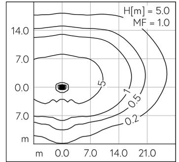
LED 3000 K 33 W 3409 lm-h H = 4.5 m / CIE Flux 22 59 90 100 100 / A10 selon DIN...
