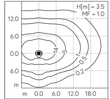
LED 3000 K 33 W 3409 lm-h H = 3.5 m / CIE Flux 22 59 90 100 100 / A10 selon DIN...
