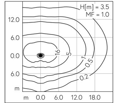
LED 4000 K 33 W 3741 lm-h H = 3.5 m / CIE Flux 23 57 89 100 100 / A10 selon DIN ...
