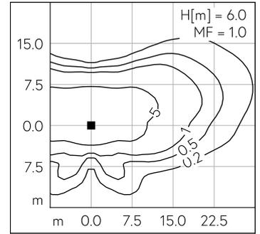
LED 3000 K 25.5 W 3756 lm-h H = 5 m / CIE Flux 35 69 94 100 100 / A30 selon DIN...
