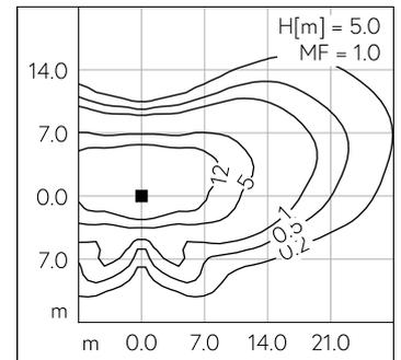
LED 3000 K 34 W 4645 lm-h H = 5 m / CIE Flux 35 69 94 100 100 / A30 selon DIN 5...
