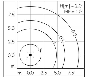
LED 3000 K 14.3 W 695 lm-h H = 2 m / CIE Flux 15 39 67 56 100 / C11 selon DIN 5040
