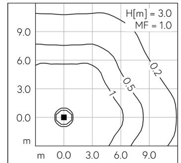
LED 3000 K 13.6 W 982 lm-h H = 3 m / CIE Flux 12 37 66 55 100 / C11 selon DIN 5040
