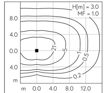
LED 4000 K 44 W 5856 lm-h H = 3 m / CIE Flux 41 78 96 100 100 / A30 selon DIN 5...
