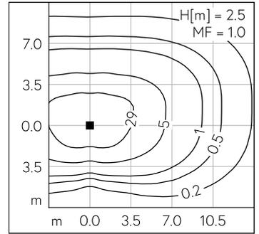
LED 3000 K 44 W 5704 lm-h H = 3 m / CIE Flux 41 78 96 100 100 / A30 selon DIN 5...
