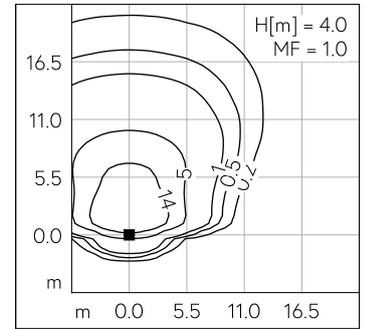
LED 3000 K 14.6 W 2010 lm-h H = 4 m / CIE Flux 32 65 94 100 100 / A20 selon DIN ...
