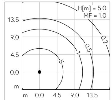
LED 3000 K 27 W 2827 lm-h H = 5 m / CIE Flux 38 67 86 92 100 / A31 selon DIN 5040
