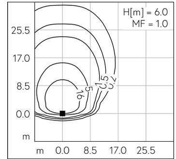
LED 3000 K 67 W 9994 lm-h H = 6 m / CIE Flux 35 72 95 100 100 / A30 selon DIN 5...
