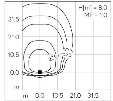
LED 3000 K 51 W 7692 lm-h H = 8 m / CIE Flux 37 74 96 100 100 / A30 selon DIN 5...
