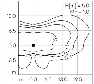
LED 3000 K 37.6 W 4692 lm-h H = 5 m / CIE Flux 34 68 94 100 100 / A20 selon DIN ...
