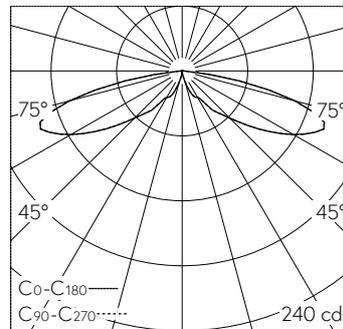
LED 4000 K 19 W 455 lm-h 98°/98° / CIE Flux 11 41 84 99 100 / A10 selon DIN 5040
