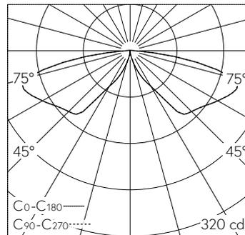
LED 4000 K 28 W 798 lm-h 70°/70° / CIE Flux 15 47 82 99 100 / A10 selon DIN 5040
