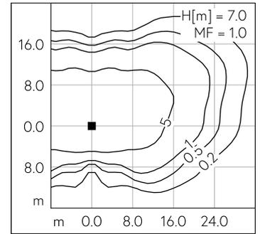
LED 4000 K 53 W 7770 lm-h H = 7 m / CIE Flux 33 71 97 100 100 / A20 selon DIN 5...
