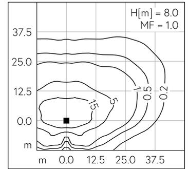
LED 3000 K 206 W 28914 lm-h H = 8 m / CIE Flux 32 65 92 100 100 / A20 selon DI...
