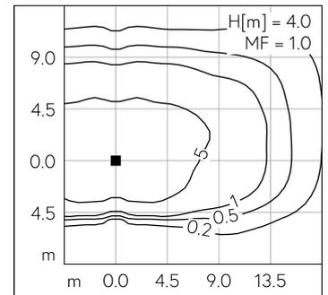
LED 4000 K 18.4 W 2474 lm-h H = 4 m / CIE Flux 38 75 96 100 100 / A30 selon DIN ...
