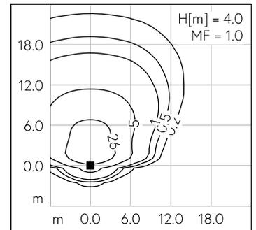
LED 3000 K 52 W 7174 lm-h H = 4 m / CIE Flux 32 67 95 100 100 / A20 selon DIN 5...
