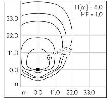
LED 4000 K 134 W 19831 lm-h H = 7 m / CIE Flux 35 71 95 100 100 / A30 selon DIN ...
